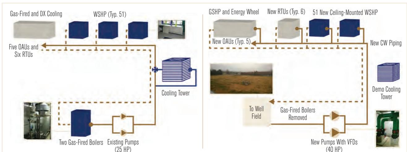
FIGURE 1A (LEFT) Existing oversized WSHPs, aged OAUs, and RTUs consumed more energy and generated maintenance challenges. FIGURE 1B (RIGHT) The upgraded HVAC system features higher efficiency GSHPs and OAUs, which eliminated the need for existing cooling towers and gas-fired boilers.
